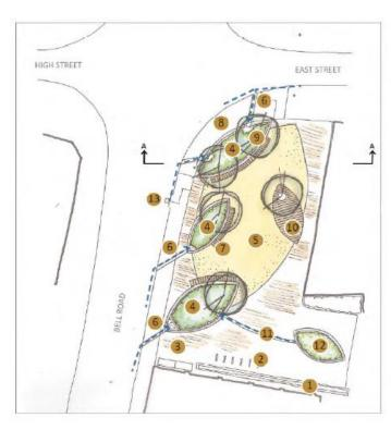
Storage attenuation for stormwater provided in large bioretention planters and sub-base storage below new permeable paving informal shapes reminiscent of large leaves as 'green infrastructure' features and historic Sittingbourne barges create focal point with integrated seating.
